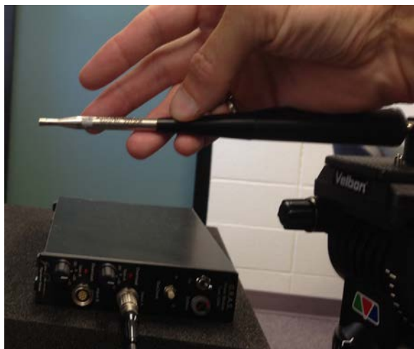
Figure 7: GRAS type 46DP 1/8" microphone and type 12AA power supply.
