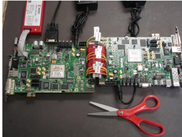
Prototype System IO Bus Implemented with Wires between two Virtex-5 FPGAs
