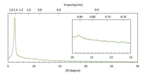
Figure S1. XRD pattern of archetypical FAU-ZTC.
