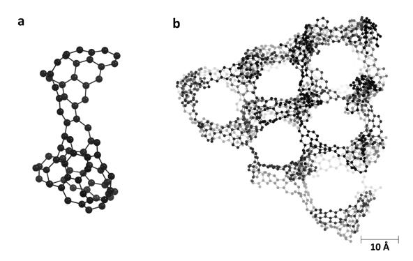
**Figure S14.** Nishihara Model II (2018): (a) a representative two-cell open-blade subunit (out of 36 different subunits within the  $2 \times 2 \times 2$  supercell) and (b) an extended multi-cell structure. Hydrogen is excluded for clarity.
