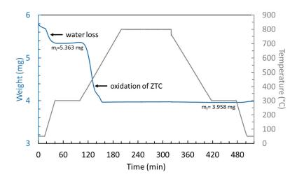
**Figure S3.** Thermal gravimetric analysis of archetypical FAU-ZTC. Three regions of weight loss are observed: water loss at 50 °C during purge (0-12 min), water loss between 50-300 °C (12-42 min), and oxidation of ZTC above 300 °C (87-158 min).
