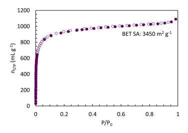
Figure S2. Equilibrium  $N_2$  adsorption/desorption isotherm of archetypical FAU-ZTC at 77 K (filled/unfilled, respectively).
