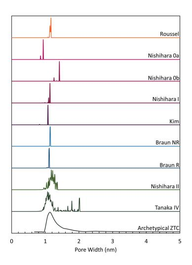
**Figure S4.** Experimental and theoretical N<sub>2</sub>-accessible pore-size distributions for all periodic **FAU**-ZTC models and archetypical **FAU**-ZTC.
