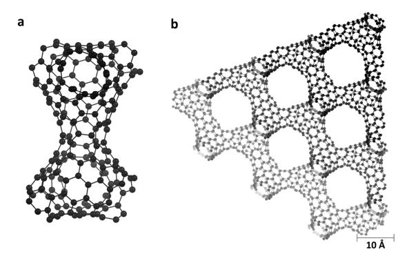
**Figure S18.** Braun Model R (2018): (a) tetrahedrally-coordinated, negatively curved "closed-strut" subunit and (b) an extended multi-cell structure, after structural relaxation.
