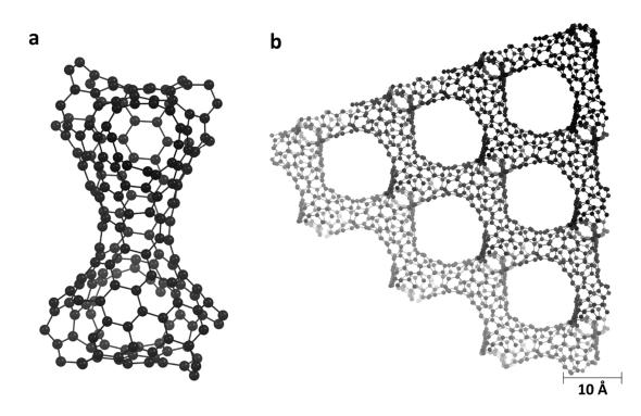
**Figure S17.** Braun Model NR (2018): (a) tetrahedrally-coordinated, negatively curved "closed-strut" subunit and (b) an extended multi-cell structure.
