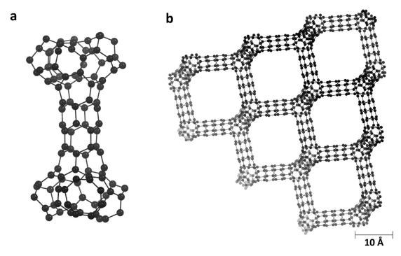
**Figure S7.** Nishihara Model 0b (2009): (a) a two-cell closed-strut subunit and (b) an extended multi-cell structure.
