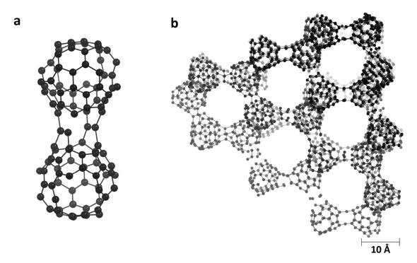
**Figure S10.** Nueangnoraj Model (2013): (a) a two-cell closed-strut fullerene-like subunit and (b) an extended multi-cell structure.
