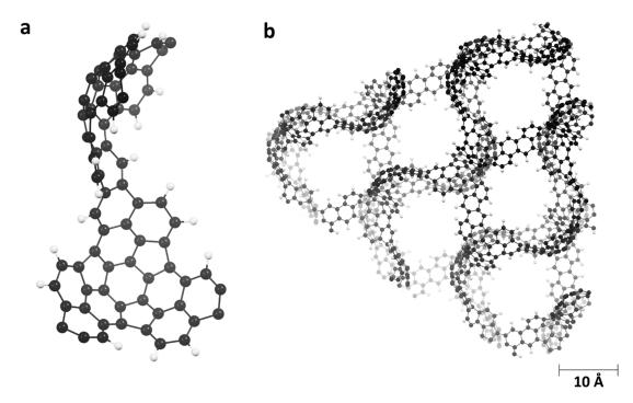
**Figure S9.** Nishihara Model I (2009): (a) a two-cell open-blade "buckybowl" subunit and (b) an extended multi-cell structure. Hydrogen is shown in white.
