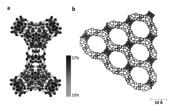
**Figure S12.** Kim Model (2016): (a) tetrahedrally-coordinated "closed-strut" subunit with partial occupancy on each lattice site (probability of occupation indicated by shading from dark grey, 22%, to white, 10%) and (b) an extended multi-cell structure.
