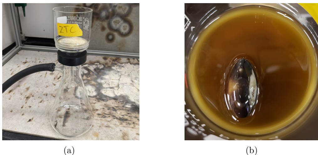
Figure B.3: FA-Zeolite Composite Filtration; (a) Vacuum-filtration set-up with designated “ZTC” Büchner funnel and (b) FA with FA-zeolite composite and stir bar poured onto the Büchner funnel filter frit.
