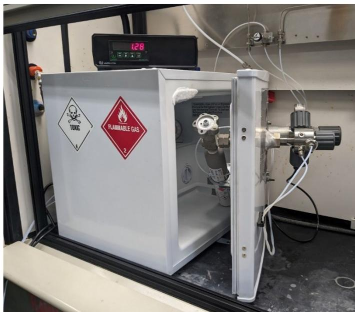
Figure S3. Experimental apparatus for storage and delivery of diborane: lecture bottle containing the B<sub>2</sub>H<sub>6</sub>/H<sub>2</sub> mixture (center) within a freezer held at -20 °C, a purgeable regulator (right), pressure transducer controller (top center), and purge, vent, and delivery gas lines (right and top right) inside a fume hood.
