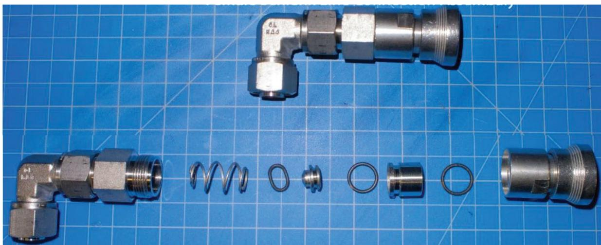
Figure A4. Female Schlenk adapter. The assembled Schlenk adapter can be seen on the top and the exploded view on bottom. The O-rings often need to be changed to achieve an acceptable seal; from left to right the valve O-ring (VT-7-OR-012, Swagelok), insert O-ring (K-FC-75-OR-015, Swagelok), and stem seal O-ring (VT-7-OR-014, Swagelok) can be seen.
