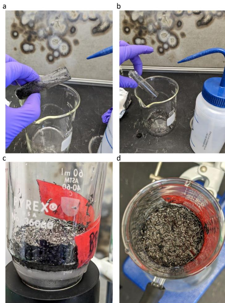
Figure A6. Collection and washing of synthesized material. (a–b) The material is collected with deionized water. (c–d) the collected material is washed over a filter frit.
