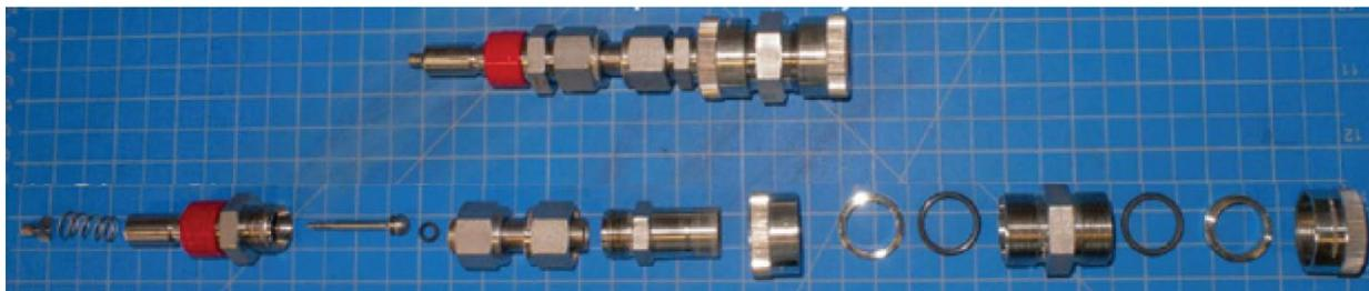
Figure A3. Male  $\frac{3}{4}$  inch Schlenk adapter. The assembled Schlenk adapter can be seen on top and the exploded view on bottom. The O-rings often need to be replaced to achieve an acceptable seal. The small stem O-ring (k-EP-70-OR-008, Swagelok) can be seen on the left, and the two Ultra-Torr O-rings (VT-7-OR-116, Swagelok) can be seen on the right of the assembly.
