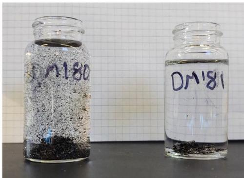
Figure S13. Two solid products generated by the pyrolysis of  $B_2C_{10}H_{14}$  (NDB) at 800 °C (route IV) can be seen: a suspension of flakes (left) and the remaining mound of the majority solid (right).
