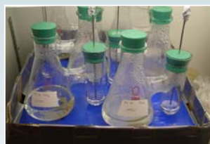
Figure 3. Biometra flasks on a shaker table inside the illuminated incubator.
