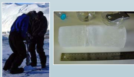
Figure 2. a. Ice cores were collected using a 10cm siple corer from both contaminated and uncontaminated areas of the Lake Fryxell ice cover. Cores were extruded into flat wrap, stored in core tubes and returned to MSU for processing. Cores used in the experiments were scraped inside a -20°C walk-in freezer using razor blades and clean techniques to remove any outside contaminants that may have been found on the surface of the cores. Several core sections were compiled to provide enough material for experiments (typically ~1500mls with a sediment weight of 2g/L).
