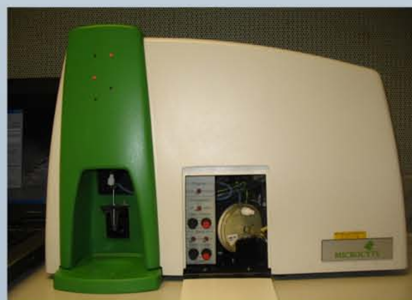
Figure #2. The Microcyte Flow Cytometer uses a laser and an infrared detector to measure particle size and concentration. It can be used to detect both sediments and microbes.
