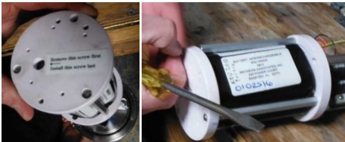
Figure 12. Cover on back of data logger assembly which holds the Lithium battery secure.
