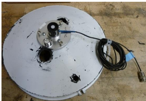
Licor LI-190SA ambient sensor with levelling fixture.
