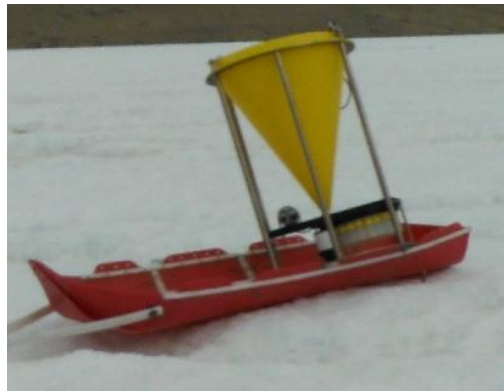
Figure 6. A sled used to transport the sediment trap between the ice hole and the Polarhaven.
