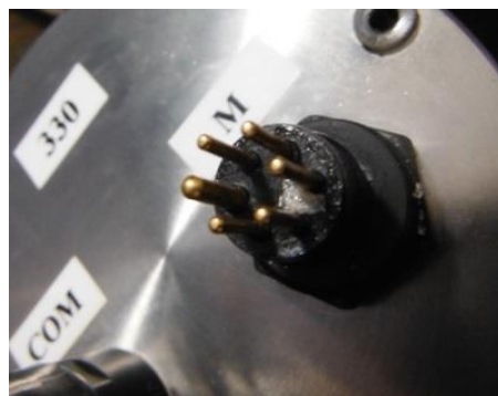
Figure 17. Connection port on the sediment trap data logger for connection to the motor.
