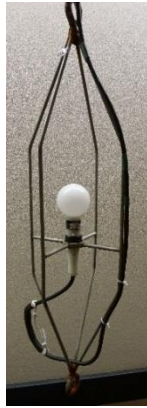
Licor LI-193SA UW sensor with lowering frame.
