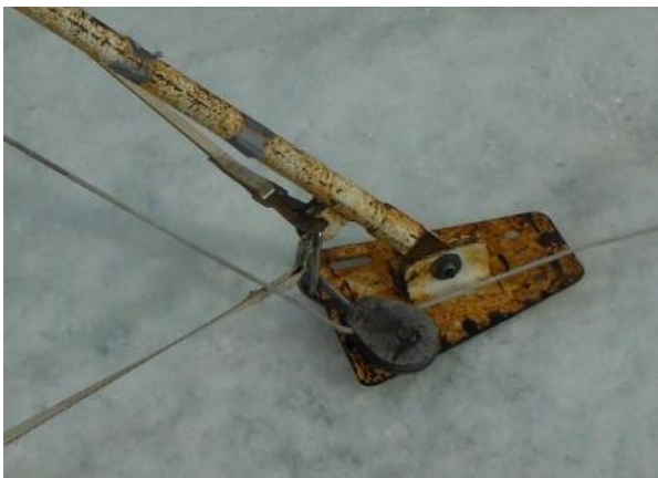
Figure 2. Set-up of the tripod used for retrieving and re-deploying the sediment trap. The end of the line marked by 'A' is to be attached to the ATV; the end of the line marked by 'B' is to be attached to the sediment trap. In this photo, the traps have already been removed. They will be re-deployed and attached to the pallet, which can be seen to the side of the hole.
