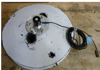
Licor LI-190SA ambient sensor with levelling fixture.
