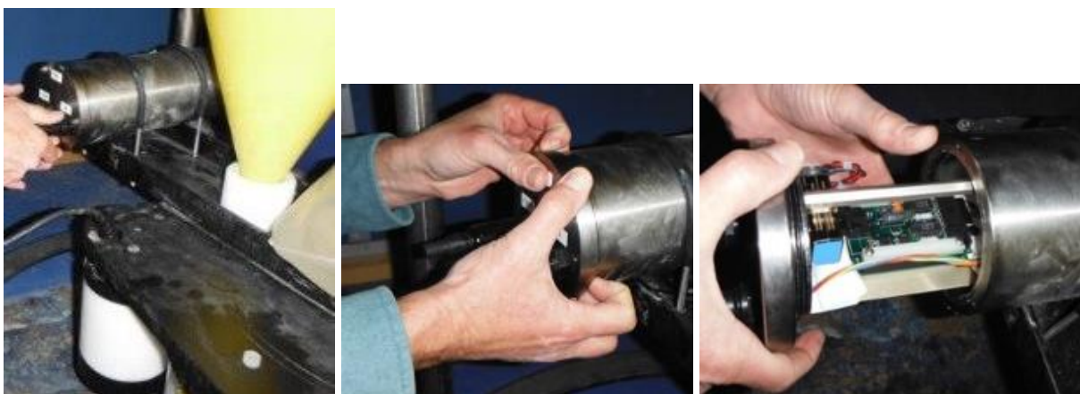
Figure 10. Removal of the cover from the sediment trap datalogger in order to access the Lithium battery.
