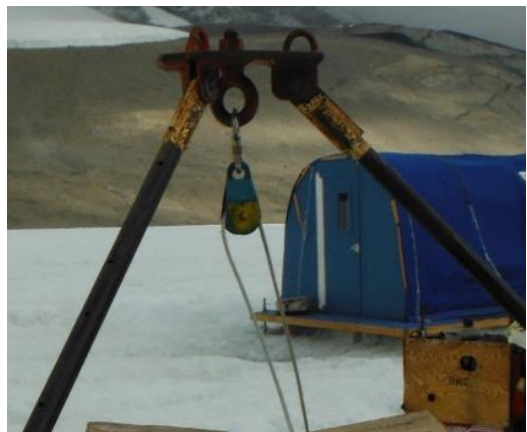
Figure 2. Set-up of the tripod used for retrieving and re-deploying the sediment trap. The end of the line marked by 'A' is to be attached to the ATV; the end of the line marked by 'B' is to be attached to the sediment trap. In this photo, the traps have already been removed. They will be re-deployed and attached to the pallet, which can be seen to the side of the hole.
