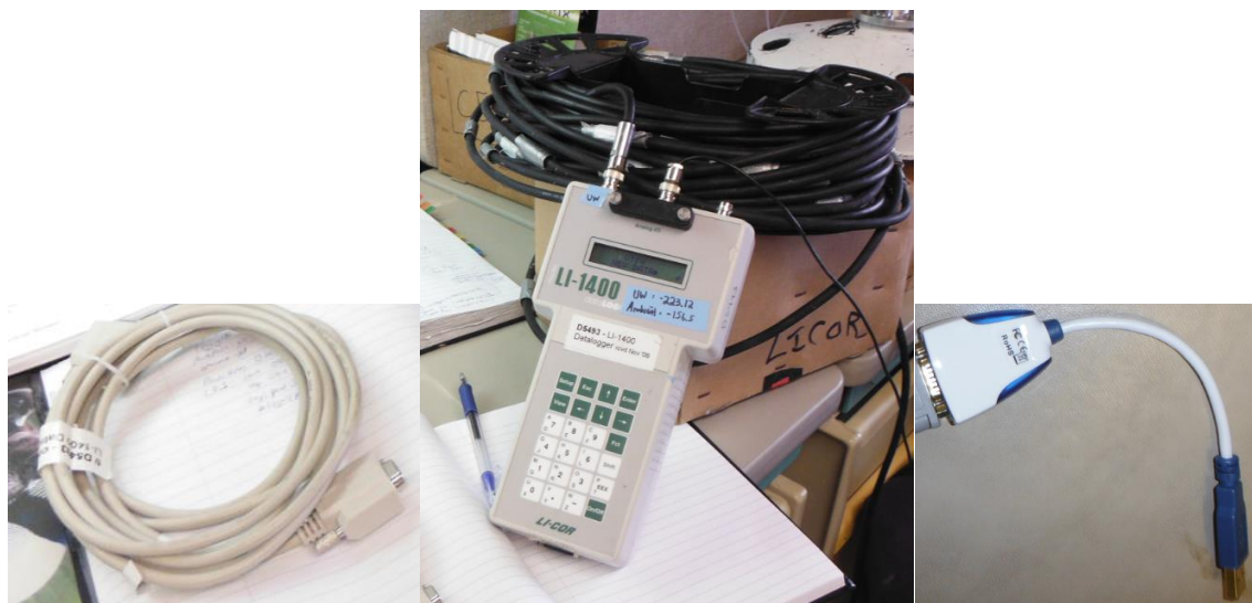
Licor LI-1400 Data Logger with 30m underwater cable. Downloading cable (left) and USB converter (right).
