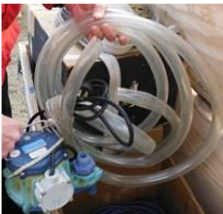
Figure 4. The peristaltic pump used to pump the water from the funnel of the sediment trap upon retrieval from lake.
