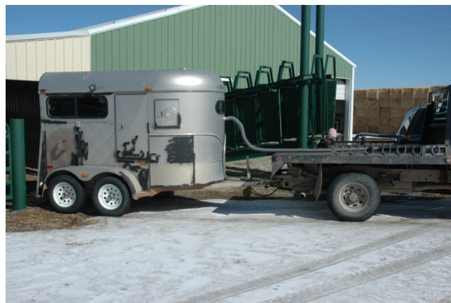
Figure 1: This horse trailer adapted as an indirect calorimetry system for measuring rate of oxygen consumed and carbon dioxide produced by cattle.
