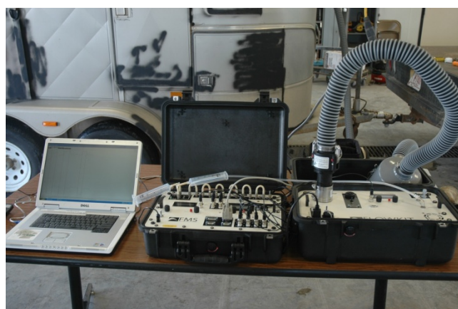
Figure 2: A field metabolic system from Sable Systems, Las Vegas, NV, USA) hooked up to a horse trailer and used for measuring rate of oxygen consumed and carbon dioxide produced for cattle confined to a horse trailer.
