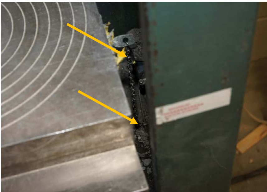
Fig. 5.6: Chain Connected to Limit Switch of Hydraulic Piston. (Before use, make sure limit switch and chain are not obstructed or jammed.)
