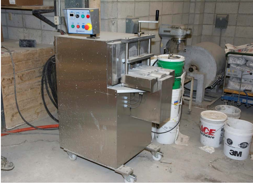
Fig. 7.15: GeneQ Inc. Concrete Grinder
