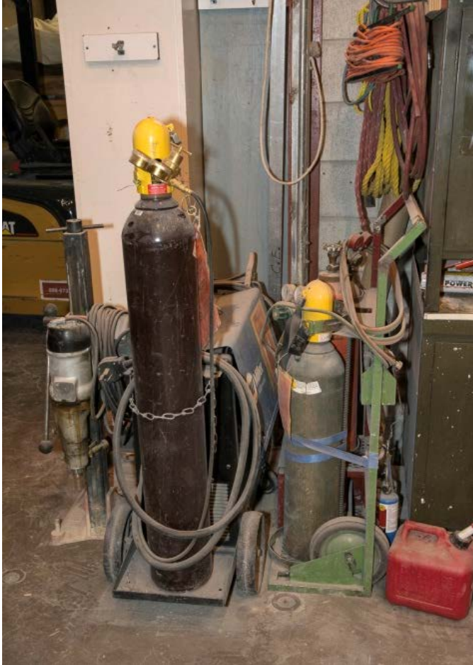
Fig. 6.6: Welder and Cutting Torch
