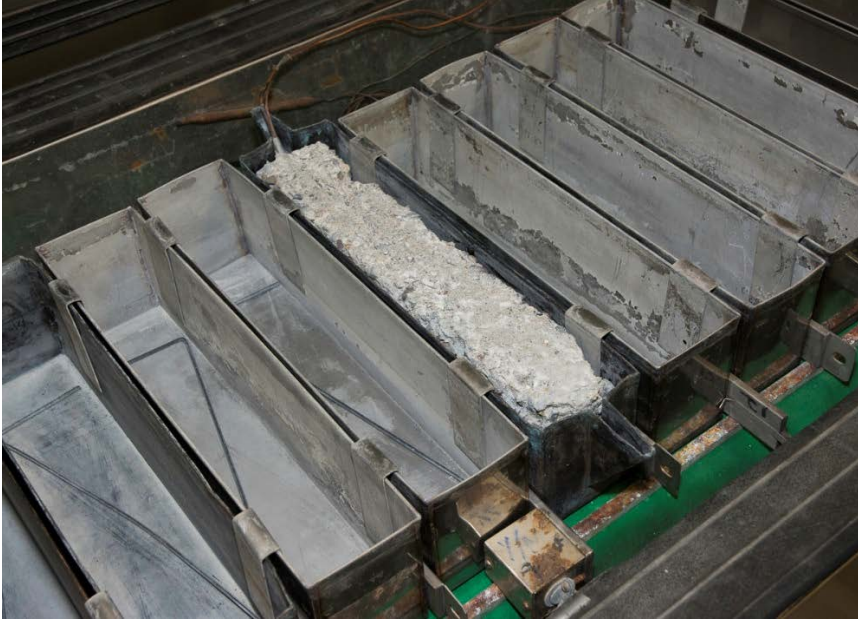
Fig. 5.10: Concrete Freezer with Temperature Reference Specimen
