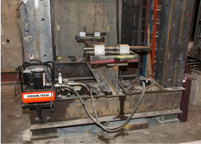
Fig. 6.8: Hydraulic Drive of Load Frame
